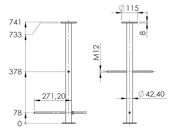
1 – Dig holes with a depth of 750 mm. For most types of soil the dimensions of the hole should be 500x500x750mm.
