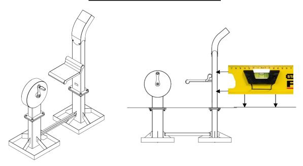
The installation frames are designed in such a way that no liquid concrete is necessary, just cover the frame with the soil. When the ground contains lots or only sand, then we advise to use liquid concrete.
