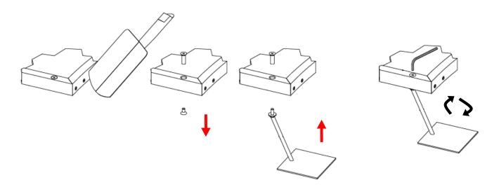
Attaching the anchor pin on each corner:
